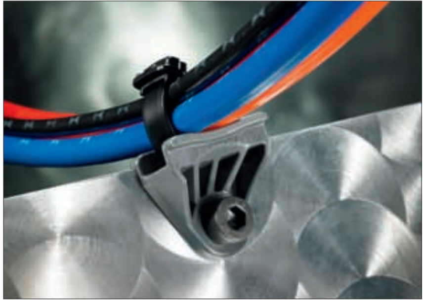
Axial oval mounts stand off bundles from frame rails and cross members to prevent them from rubbing and chafing.
