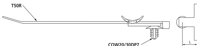
COW Clip with Cable Tie Assembly
