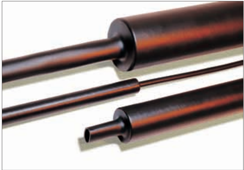
Medium wall tubing MA47 with shrink ratio 4:1 and adhesive liner.
