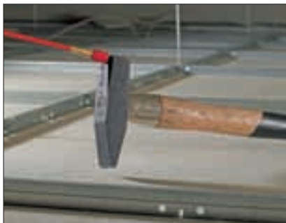
The double magnet can retrieve lost tools up to a weight of 2.5 kg.
