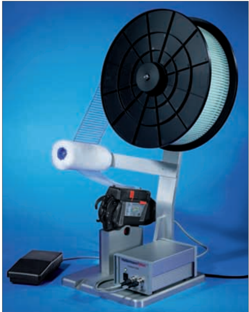
Assembly equipment, band reel, Autotool 2000 in receptacle and power supply unit.
